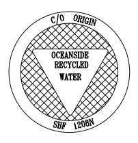
COVER WITH CITY OF OCEANSIDE WATER DEPT. CASTED ON TOP BY SOUTH BAY FOUNDRY FRAME AND COVER (SBTT)
