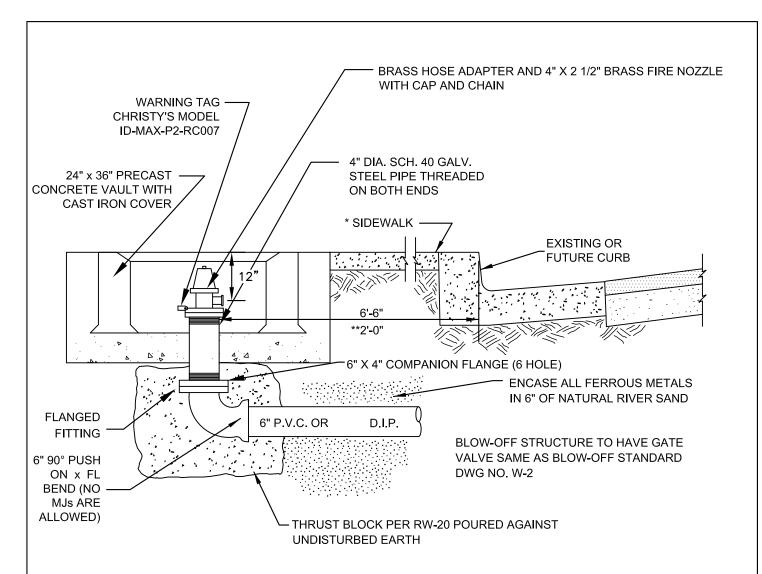
\* NOTE: ON TEMPORARY DEAD END STREETS THE BLOW-OFF SHALL BE PLACED BEHIND THE BARRICADE
