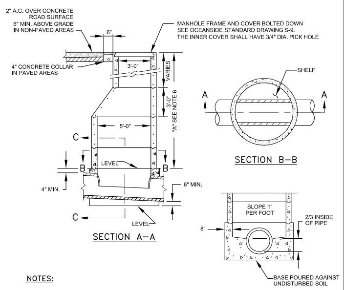
1. MANHOLE FRAME AND ALL JOINTS SHALL BE SET IN CLASS "C" MORTAR, 3/8" THICK, NEATLY STRUCK READY-TO-USE PLASTIC JOINT SEALING COMPOUND AND PRIMER. (ALSO SEE NOTE 6 BELOW).
